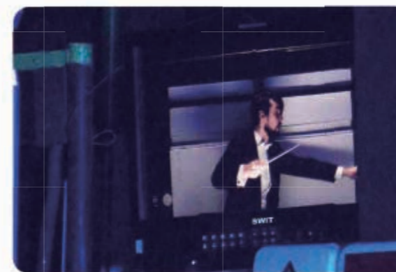
Zero Latency 4K monitor used in Baltic Opera, Poland, can display the live video feed from the orchestra pit in real time, allowing performers to follow the conductor's gestures with perfect synchronization.
