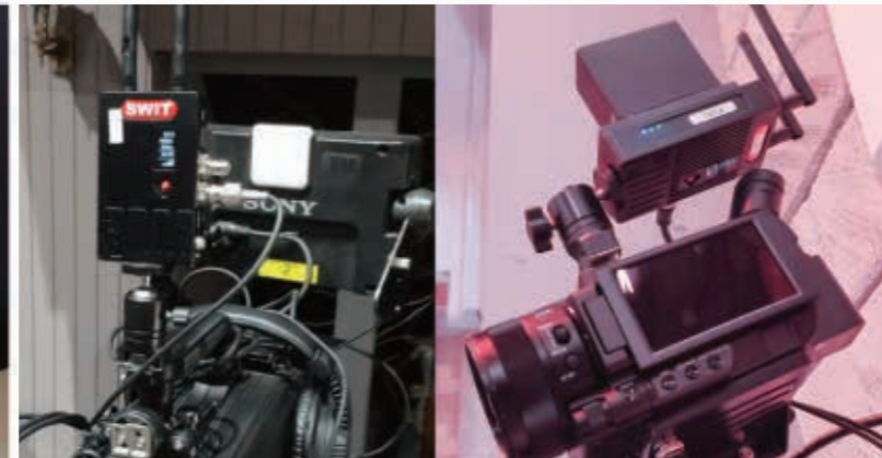
The FLOW wireless Tx fits for different kinds of cameras by SDI or HDMI
