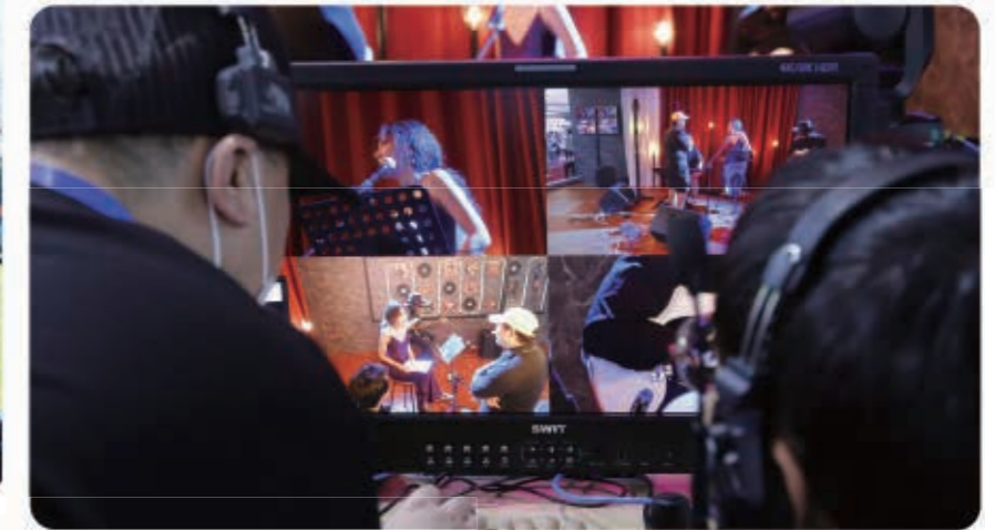
The 31.5-inch Local Dimming 4K HDR monitor, 1,000,000:1 ultra contrast for high level live productions with 4x 12G-SDI quadview.
