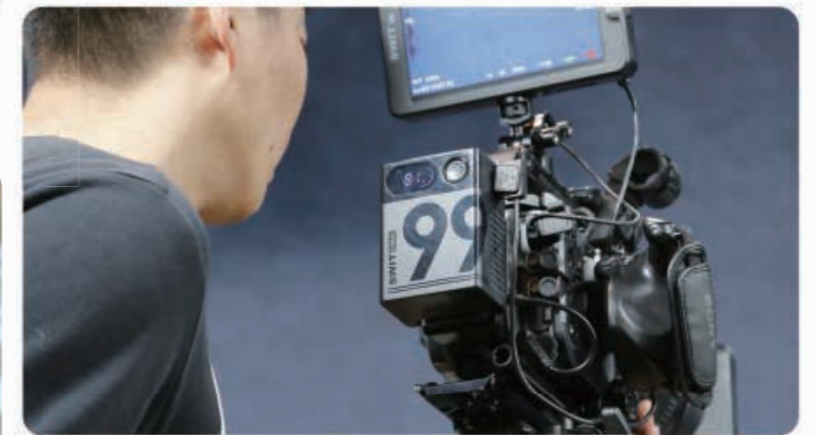
The 99Wh pocket V-mount battery with 65W USB-C, D-tap, DC barrel, info display, and 150W constant high power.
